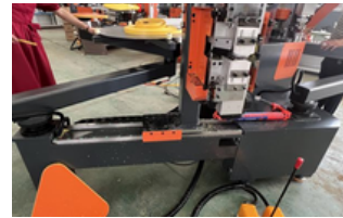
Edge excess scraping straight panels
