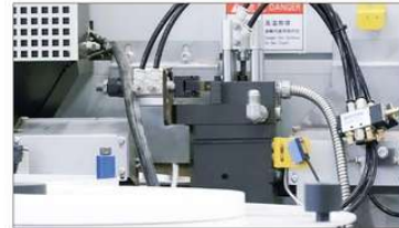
Easy to clean PUR glue reservoir is optional
