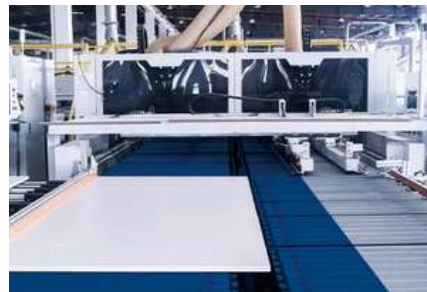
Parts above 650mm can be processed with both drill banks on one table
