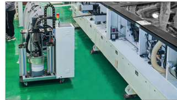
Pur adhesive melting unit available for water-proof and zero joint requirements
