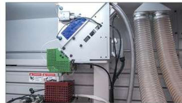
Automatic glue refill device available
