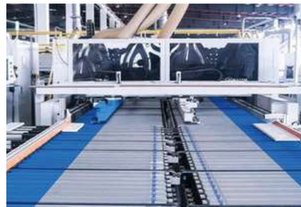
Parts under 650mm can be processed on two tables simultaneously
