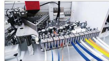
2/4/6/12 slot servo tape magazines available for upgrade. Smooth guidance, servo driven, the edge infeed is both precise and swift
