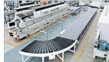
Edgebander with return conveyors, greatly helps reducing down time while improving productivity
