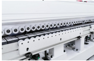
Beam gantry with roller pressure system
